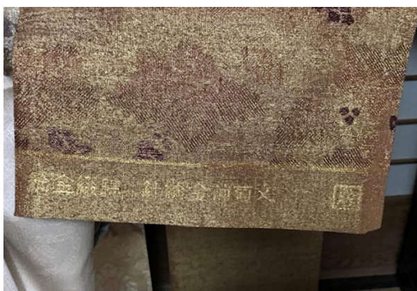
Picture 14 & 15 – Fabric woven out of Nenkin-Shi Yarns
